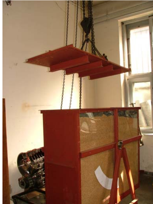
Fig. 7. Stiffening of the hatch cover
