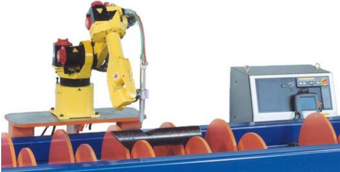
Fig. 7. Robot Saddle and Hole Cutting Machine
