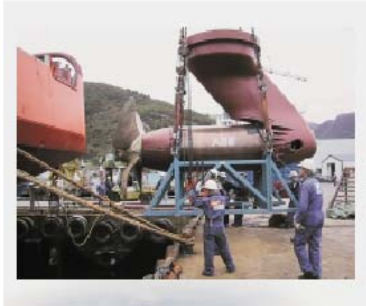
Slika 17 Compact Azipod® spreman za ugradnju Fig. 17 Compact Azipod® prepared for fitting
