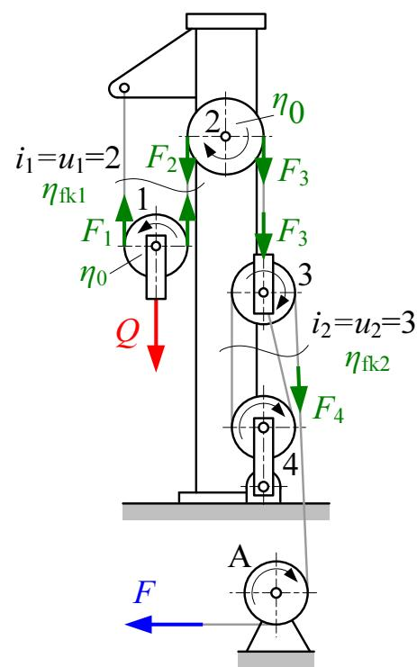
$$\left. \begin{array}{l} F_1 = F_2 \cdot \eta_0 \\ Q = F_1 + F_2 \end{array} \right\} \quad F_2 = \frac{Q}{1 + \eta_0}$$
