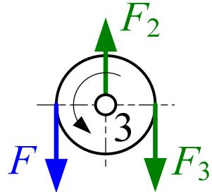
$$\left. \begin{array}{l} F + F_3 = F_2 \\ F > F_3 \quad \Rightarrow \quad F_3 = F \eta_0 \end{array} \right\} F_2 = F(1 + \eta_0)$$
