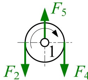
$$\left. \begin{array}{l} F_5 = F_2 + F_4 \\ F_4 > F_2 \Rightarrow F_4 = F_2 / \eta_{0,k} \end{array} \right\} F_5 = F_2 \cdot (1 + 1/\eta_{0,k})$$
