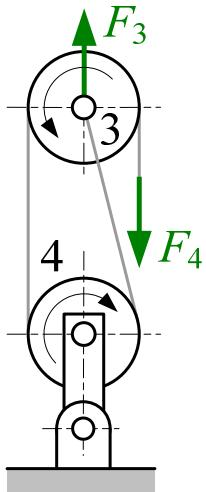
$$F_3 = \frac{Q}{(1+\eta_0) \cdot \eta_0} \quad v_8 = 6 \cdot v_2 \quad v_6 = 2 \cdot v_2$$
