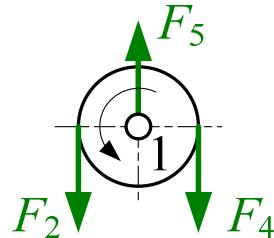
$$\left. \begin{array}{l} F_5 = F_2 + F_4 \\ F_2 > F_4 \Rightarrow F_4 = F_2 \cdot \eta_0 \end{array} \right\} F_5 = F_2 \cdot (1 + \eta_0)$$
