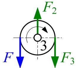
$$\left. \begin{array}{l} F + F_3 = F_2 \\ F_3 > F \quad \Rightarrow \quad F_3 = F/\eta_{0,k} \end{array} \right\} F_2 = F \cdot \left( 1 + 1/\eta_{0,k} \right)$$
