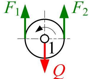
$$\left. \begin{array}{l} F_2 > F_1 \Rightarrow F_1 = F_2 \cdot \eta_0 \\ Q = F_1 + F_2 \end{array} \right\} F_2 = \frac{Q}{1 + \eta_0}$$
