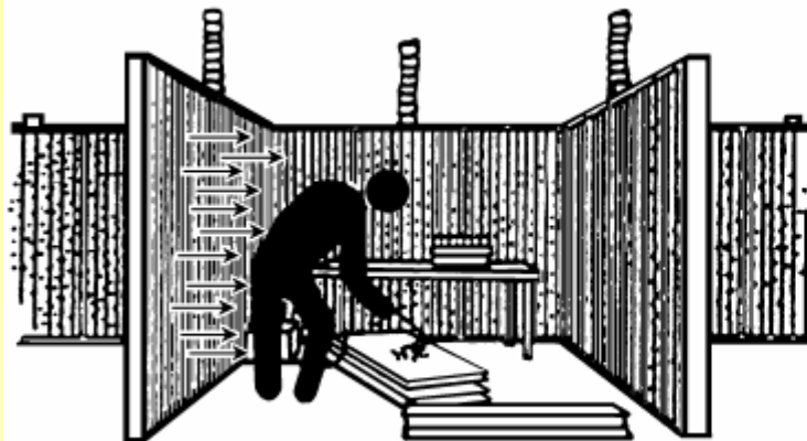
B. AIR OASIS WITH HORIZONTAL AIR SUPPLY
