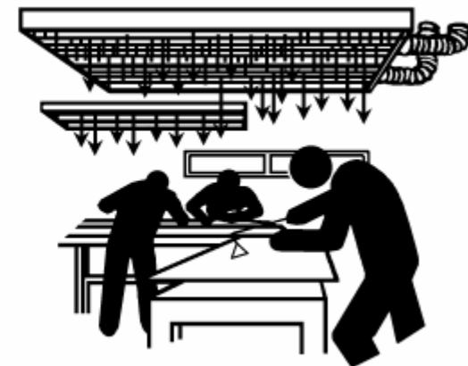
C. AIR OASIS WITH VERTICAL AIR SUPPLY
