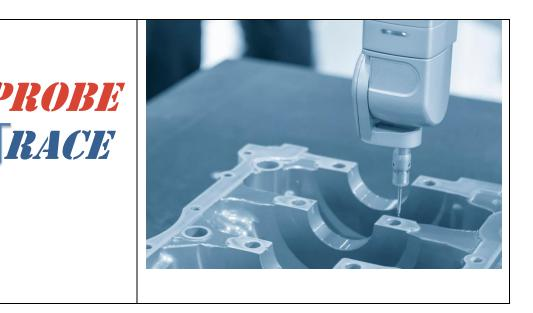
Surface texture and form of products are important features to be examined and numerically characterised as parameters for engineering and scientific purposes. Such features of surfaces have great impacts on wear resistance, bearing, sliding and lubricating properties, fatigue and corrosion resistance, functionality, etc. Form and surface measurement devices with contact probes and stylus are used to characterise such surfaces.
