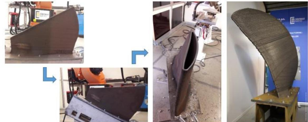
Flap rudder using lightweight and high-performance material for container ship
