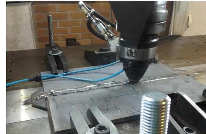
*FSP preliminary trials performed in AIMEN on homogeneous sample S690 material*
