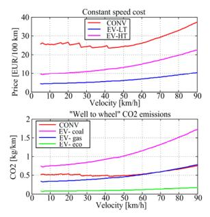
Comparative plots of constant-velocity energy cost and well-to-wheel CO2 emissions for conventional and electric trucks.
