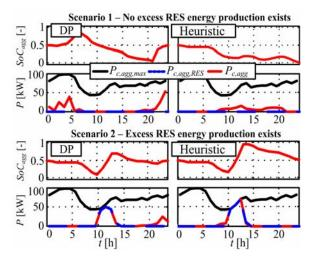
Aggregate battery charging results using DP optimization and heuristic approaches for two RES energy production scenarios.
