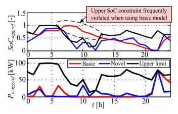
DP-optimised aggregate battery charging power and SoC daily time profiles.
