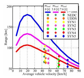
Predicted range of e-truck for constant velocity driving and various certified and synthesized naturalistic driving cycles.
