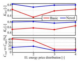
Correlation factors of basic and novel aggregate battery models for different electricity price models.
