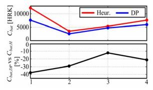
Comparative DP vs. heuristic algorithm results on aggregate battery charging costs for three months period and four electricity price models.
