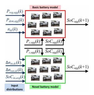
Illustration of basic and novel aggregate battery models including corresponding input distributions, control and state variables.
