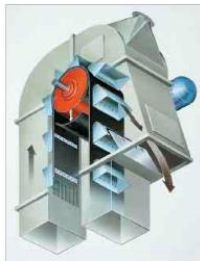
The bucket elevator head
