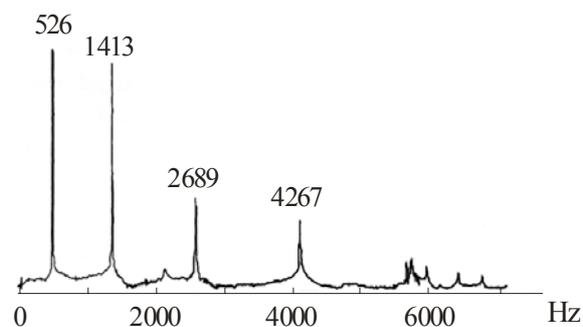
Notice that the spectrum consists of the fundamental at  $f = 526$  Hz, and of the *non-integer* partials at  $2.68f = 1413$  Hz,  $5.11f = 2689$  Hz and  $8.11f = 4267$  Hz. Such a spectrum in which the frequencies of vibration are not the integer multiples of some fundamental  $f$  is called *non-harmonic* and the corresponding sound is called *non-harmonic sound*. Since at least some partials do not repeat exactly within the period of the fundamental, harmonic sound waves are not periodic.
