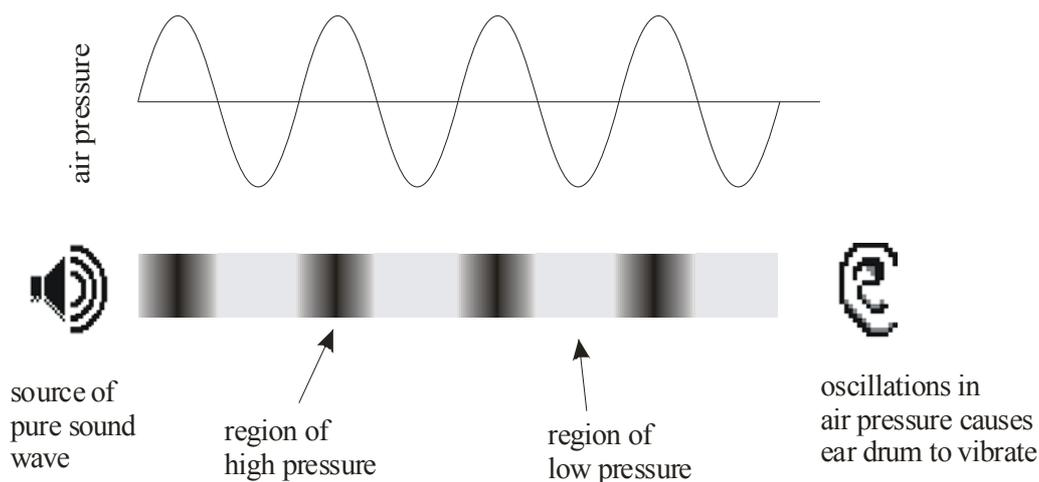
The peaks represent times when air molecules are clustered, causing higher pressure. The valleys represent times when the air density, and hence the pressure, is lower. The wave pushes against the ear drum in times of higher pressure, and pulls during times of low pressure, causing the drum to vibrate. These vibrations are perceived as sound.
