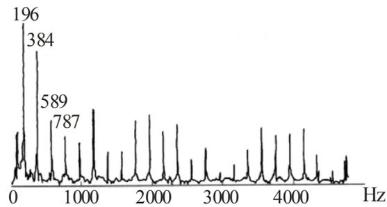
Notice that the spectrum consists of the fundamental at  $f = 196$  Hz and of the near *integer* partials at  $2f \approx 384$  Hz,  $3f \approx 589$  Hz,  $4f \approx 787$  Hz etc. Such a spectrum in which all the frequencies of vibration are integer multiples of some fundamental  $f$  is called *harmonic* and the corresponding sound is called *harmonic sound*. Since every partial repeats exactly within the period of the fundamental, harmonic sound waves are periodic.
